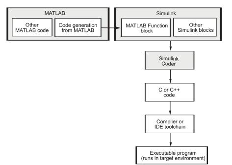
The code generation workflow is a part of the V-model for system development. The process includes code generation, code verification, and testing of the executable program in real-time. For rapid prototyping of a real-time application, typical tasks are:
